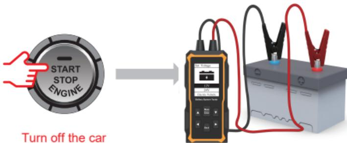
After preparations are complete, choose Batteries Test according to 5.1 . Test results are as follows:
